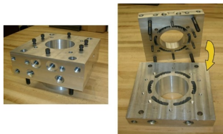
Figure 6. Cylinder block construction showing the 6 coolant passages surrounding the liner to control temperature and heat transfer
