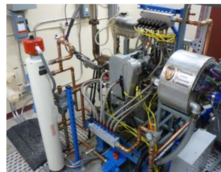
Figure 1. SCE transient test system that simulates MCE dynamic performance
